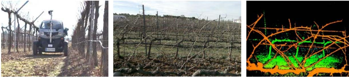
**Figure 1:** (a) Electric mobile platform comprising Kinect v2 sensor. (b) RGB section of the crop. (c) Depth image of the crop
